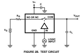
Test Circuits and Waveforms (Continued)
