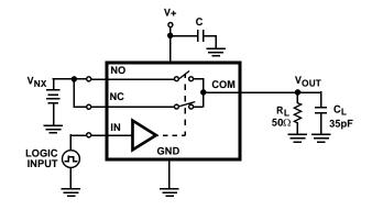
C<sub>L</sub> includes fixture and stray capacitance.
