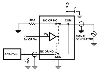
FIGURE 6. CROSSTALK TEST CIRCUIT
