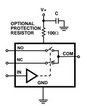
FIGURE 8. V+ SERIES RESISTOR FOR ENHANCED ESD AND LATCH-UP IMMUNITY
